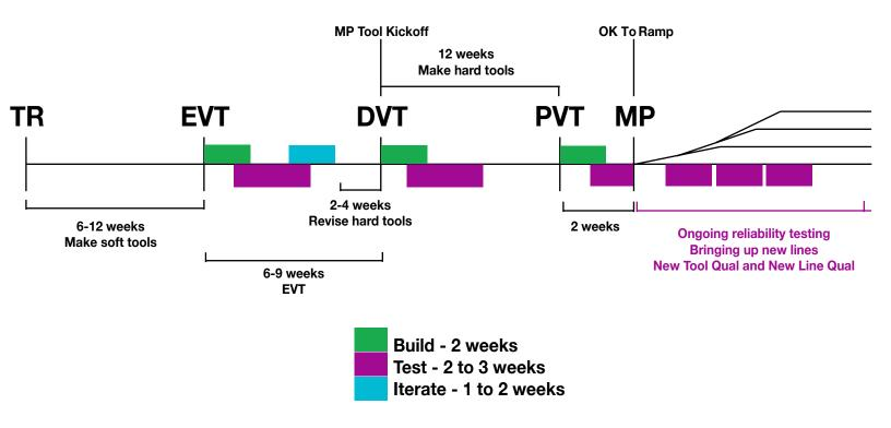
Hardware teams build their products by traversing through these phases and into mass production using the Build-Test-Iterate hardware iteration cycle.
