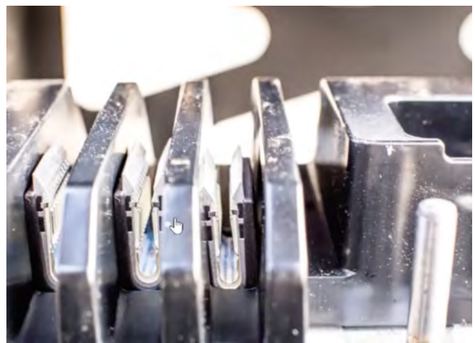
Second potential failure point: black plastic front covers installed onto module
